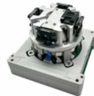
TensorADCS-10m Integrated Attitude Determination and Control System
