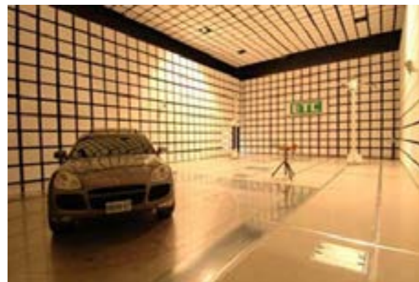
10m Anechoic Chamber
